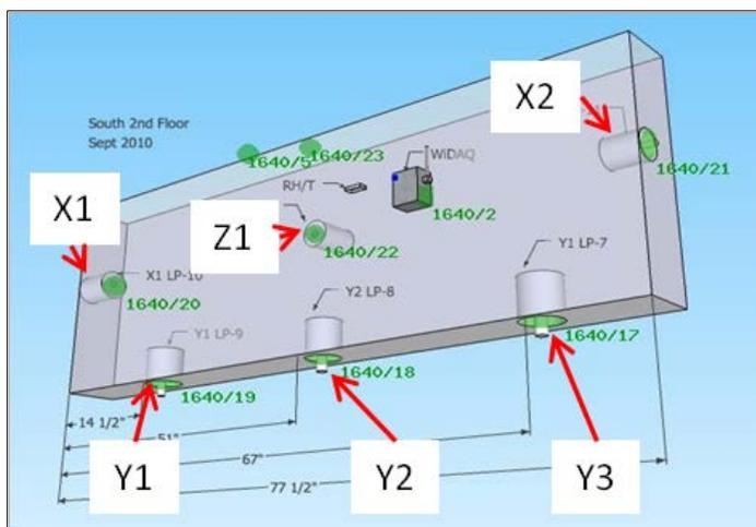
**FIGURE 13 - Sensor Location in XPS Board**
