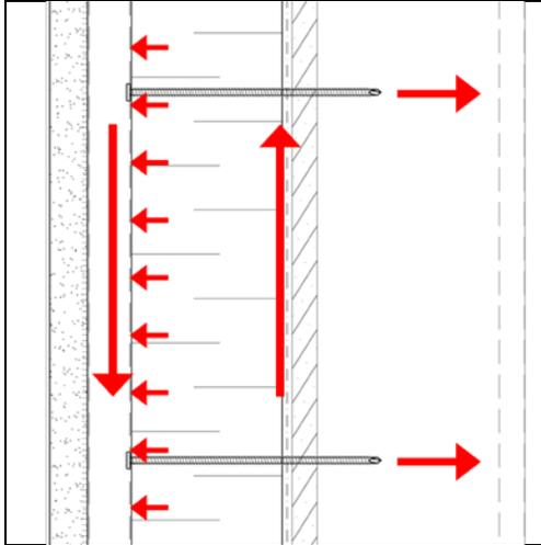
**FIGURE 7 - Insulation Cladding Force Diagram**
