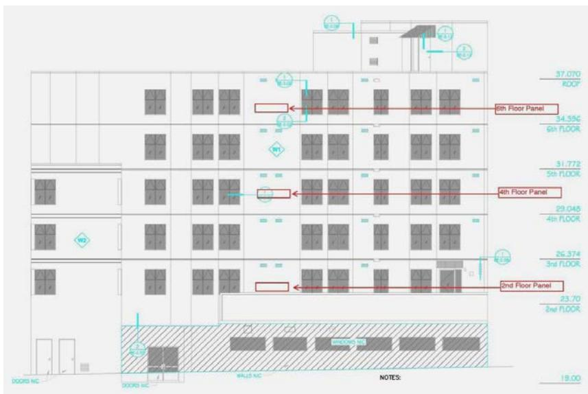
**FIGURE 11 - Measurement Panel Locations (South Elevation)**
