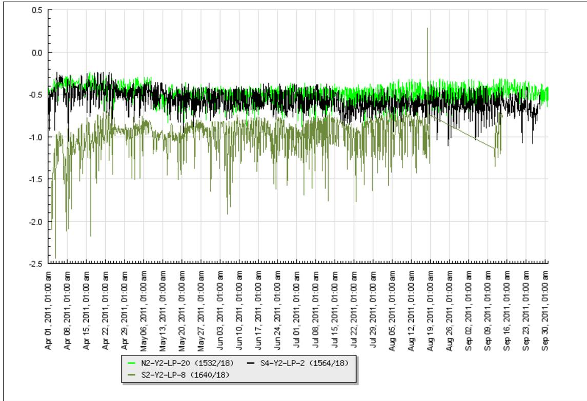
**FIGURE 21 - Vertical Displacement Measurements of North and South Panels**
