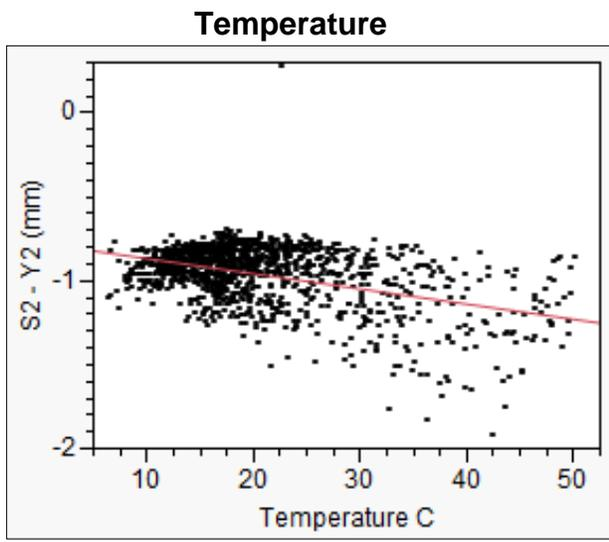
**FIGURE 24 - Y2 Displacement as Function of Temperature (2nd floor, South)**
