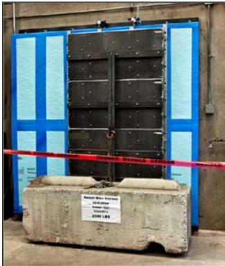
**FIGURE 8 - Load Testing Mock-up Panel**
