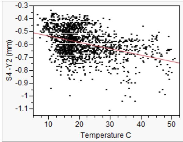
**FIGURE 25 - Y2 Displacement as Function of Temperature (4th floor, South)**
