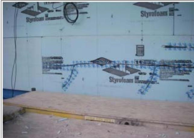
**FIGURE 16 - Measurement Panel after Installation of Displacement Sensors**
