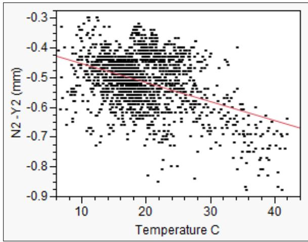
**FIGURE 23 - Y2 Displacement as Function of Temperature (2nd floor, North)**
