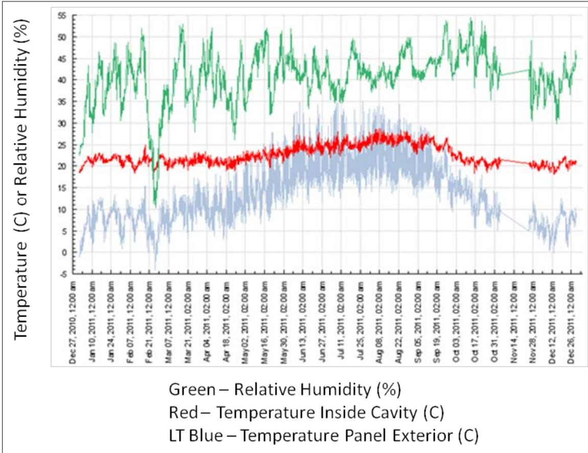
**FIGURE 28 - Temperature and Relative Humidity (2nd floor, North)**
